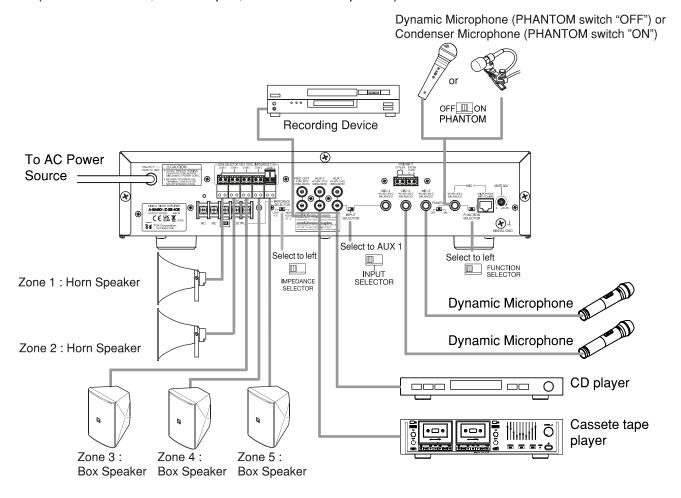
Example of External Equipment Connections (model with 5 band equalizer, 1 chime microphone, 4 microphone input, 2 aux, 1 rec out)
